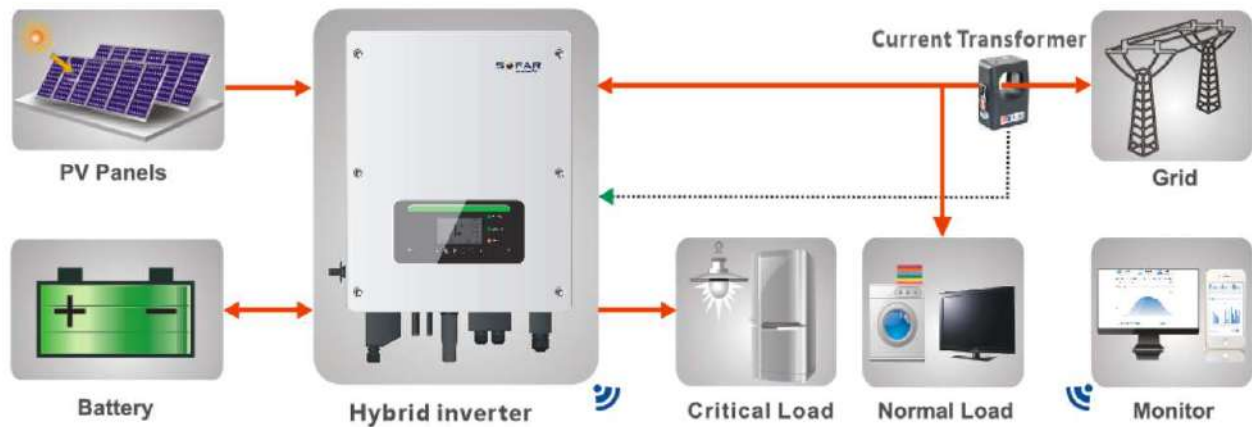
Fig. 1 HYD-ES inverter schematic diagram
