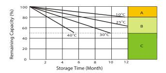
A No supplementary charge required (carrry out supplementary charge before use if 100% capacity is required)
