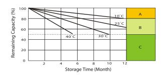
A No supplementary charge required (carrry out supplementary charge before use if 100% capacity is required)
