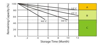
No supplementary charge required (carrry out supplementary charge before use if 100% capacity is required)
